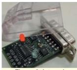
Figure 6. Internal clamshell and PCBA.
